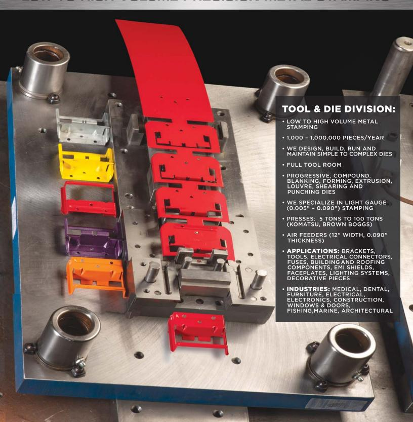
HANSEN INDUSTRIES LTD. designs, builds, runs and maintains cost-effective custom dies for producing high quality, repeatable sheet metal stamped parts.
